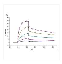
Biotinylated Human EGFR, His Tag captured on CM5 Chip via Anti-his antibody can bind Human EGF, No Tag with an affinity constant of 0.62 nM as determined in SPR assay (Biacore T200).
